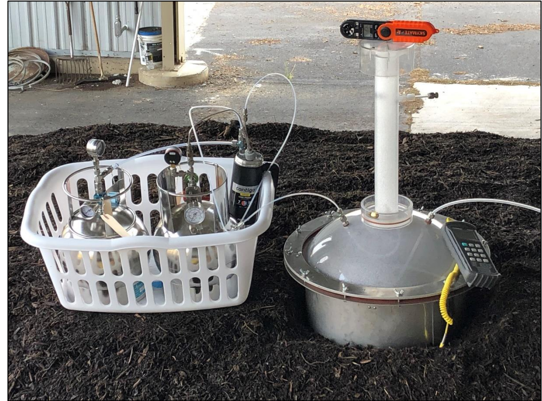
Side by side sampling from flux chamber
